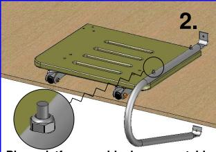
Place platform upside down on a table and drill 7/32" thru holes were the marks for the grab rail were made.
