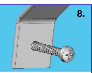
Mark the hole location of the bottom hole of the support brace then drill 3/16" pilot holes at your marks. Screw the support brace to the boat with (1) #14 x 1 1/2" screw. Apply clear silicon around the screw to seal.
