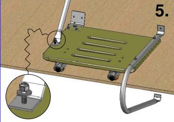
Drill 1/4" thru hole were the mark for the support bracket was made and attach the bracket to the platform with (1) 1/4-20 x 2 1/2" carriage bolt, (1) 1/4" flat washer and (1) 1/4-20 lock nut.
