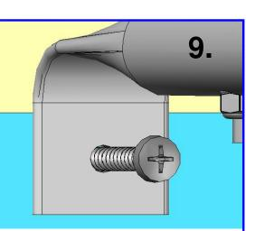
Mark the hole location of the bottom hole of the grab rail then drill 3/16" pilot holes at your marks. Screw the guard rail to the boat with (1) 14 x 1 1/2" screw. Apply clear silicon around the screw to seal.
