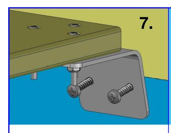
Mark the hole locations of the angle bracket on the boat then drill 3/16" pilot holes at your marks. Screw the angle bracket to the boat with (2) #14 x 1 1/2" screws. Apply clear silicon around the screws to seal.
