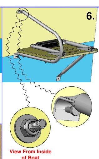
Position platform on boat and mark the upper hole of the grab rail. Drill a 1/4" thru hole at the mark. Mount the top of the grab rail to the boat with (1) 1/4-20 x 2 1/2" hex bolt, (1) 1/4" flat washer, and (1) 1/4-20 lock nut. Apply clear silicon inside the hole to seal.
