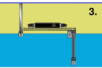
Hold the platform against the boat and find the ideal placement of the angled bracket and the support bracket. Keep in mind that the platform should be 1" from the water line and 3/4" off of the boat. Try and mount the support bracket as far aft as possible. Mark the holes on the platform.
