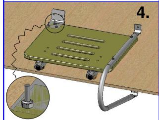
Drill (3) 7/32" thru holes were the holes for the angled bracket were marked. Countersink the top side of the holes Install the angled bracket to the platform with (3) #10-24 x 1 1/2" bolts and (3) 10-24 lock nuts.
